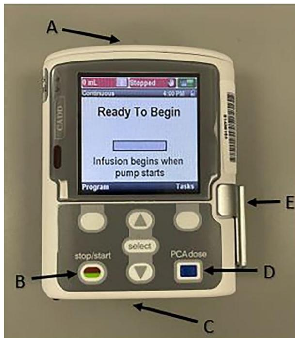
**Figure 6.** Ambulatory pump (CADD-Solis). A, Battery placement (4 AA batteries). B, Start/Stop function. C, Area of attachment between cassette and pump. D, Bolus dose button used specifically for patient-controlled analgesia. E, Latch for pump connect and disconnect.
